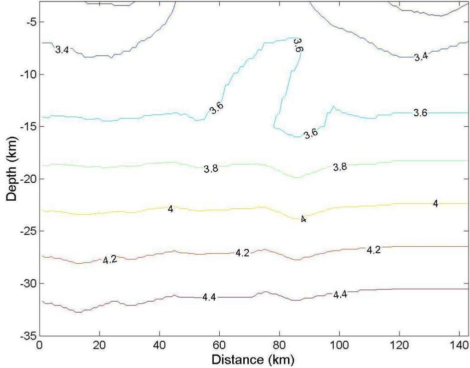
**Figure 1: Two-dimensional crustal structure for shear-wave velocities (see labels on contour lines) used for simulations. Velocities extracted from the model of Souriau and Granet (1995) along a path 42.25N-0.25E to 43.25N-1.5E.**
