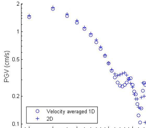
**Figure 2: Simulated peak ground velocity using the uniform (averaged up to 140km) velocity-averaged 1D structure and the true 2D structure.**
