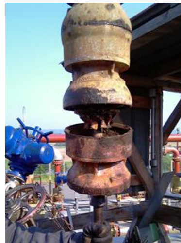
Figure 11: Status of the LSP pump after the pull operation of April 2011. Picture of the hydraulic part of the pump.
