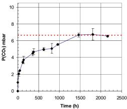
Figure 1 Example of  $CO_2$  degassing in the degassing cell. Sample from the Meuse/Haute-Marne URL (EST312 10273).  $log_{10}(PCO_2[bar]) = -2.17$  at 90 days and for a relative humidity of 95%.
