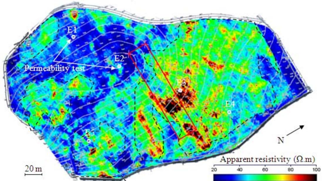
**Figure 6. Apparent electrical resistivity map obtained with the ARP technique (with a point every 0.25 m along profiles separated by 1 m). The red rectangle corresponds to the SP prospected zone. E1 to E5 correspond to permeability tests and mechanical surveys made in 2006. Topographic lines have been reported.**
