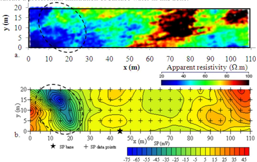
**Figure 7. a. Zoom over the ARP zone surveyed with the SP method. b. SP map obtained by kriging interpolation (with spherical model fitted to an omnidirectional variogram) of data point every 5 m (red crosses) compared to a fixed base (dark star).**
