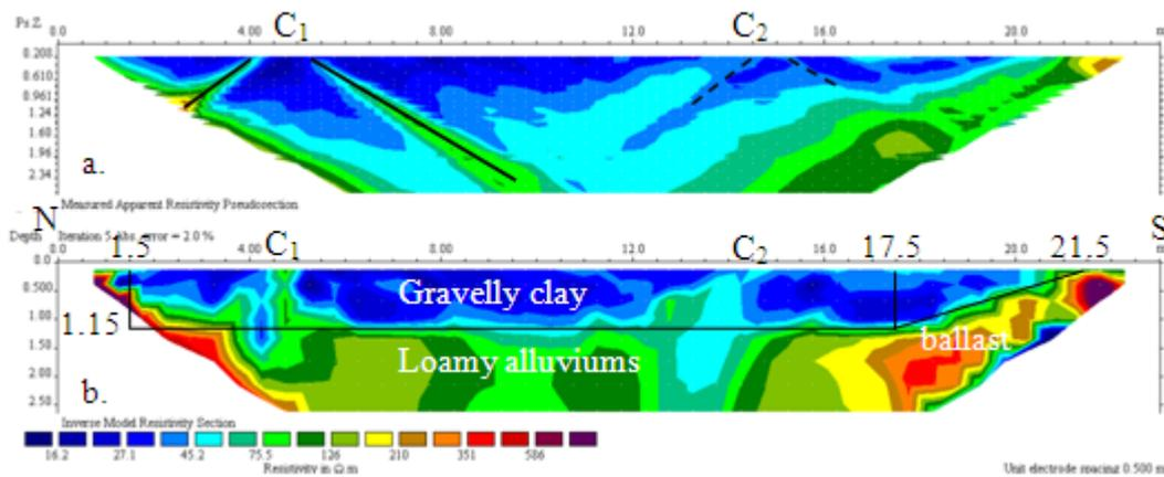
**Figure 2.** ERT<sub>1</sub> intersects the two cracks  $C_1$  and  $C_2$ . a. Measured apparent resistivity pseudosection (dipole-dipole array). b. Inverse model resistivity section (robust inversion).
