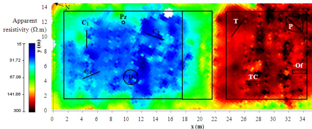
**Figure 5.** Apparent electrical resistivity map obtained with the ARP technique (with a point every 1 m in y and every 0.25 m in x direction). See Figure 4 for failures identification.
