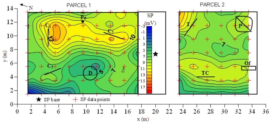
**Figure 4.** SP map obtained by kriging interpolation (with spherical model fitted to an omnidirectional variogram) of data point every 2 m (red crosses) compared to a fixed base (dark star). Failures have been reported: cracks ( $C_1$ ,  $C_2$ ,  $C_3$ ), piezometer (Pz), depression (D), tear (T), tear and crack (TC), overlap failure (Of), puncture (P).
