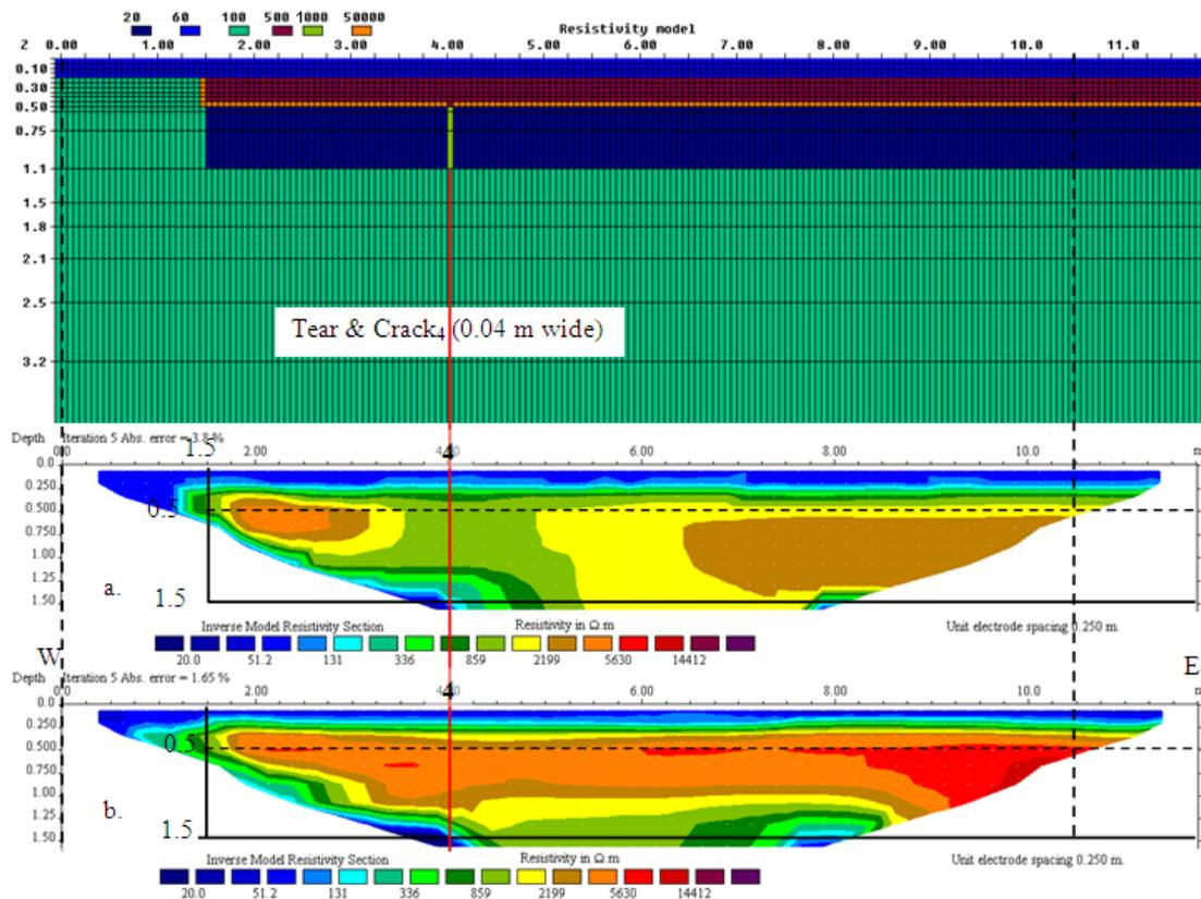
**Figure 3. a. Forward modeling of ERT<sub>2</sub> intersecting the tear of the GCL and crack of the gravelly clay (5 % noise added, wenner array, robust inversion). b. Inverse modeling of the field data (wenner array, robust inversion). Red line indicates the location of the crack and black lines the limits of the gravelly clay material.**
