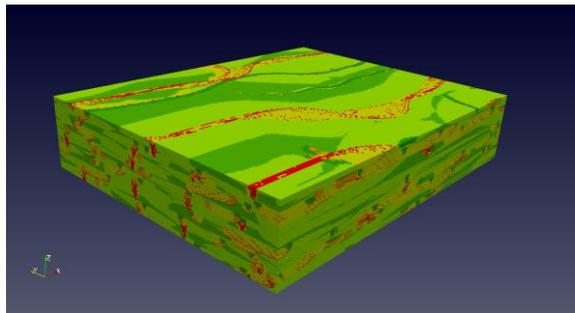
*Figure 1: 3D lithofacies block from the Flumy model. (6 million cells) There are 9 different lithofacies (cf. table 1). Relatively permeable sandy facies are represented in red and yellow (channel lags, sand plugs, point bars) whereas more impervious facies are in shades of green (overbank deposits, alluvial plain) (20x vertical exaggeration)*
