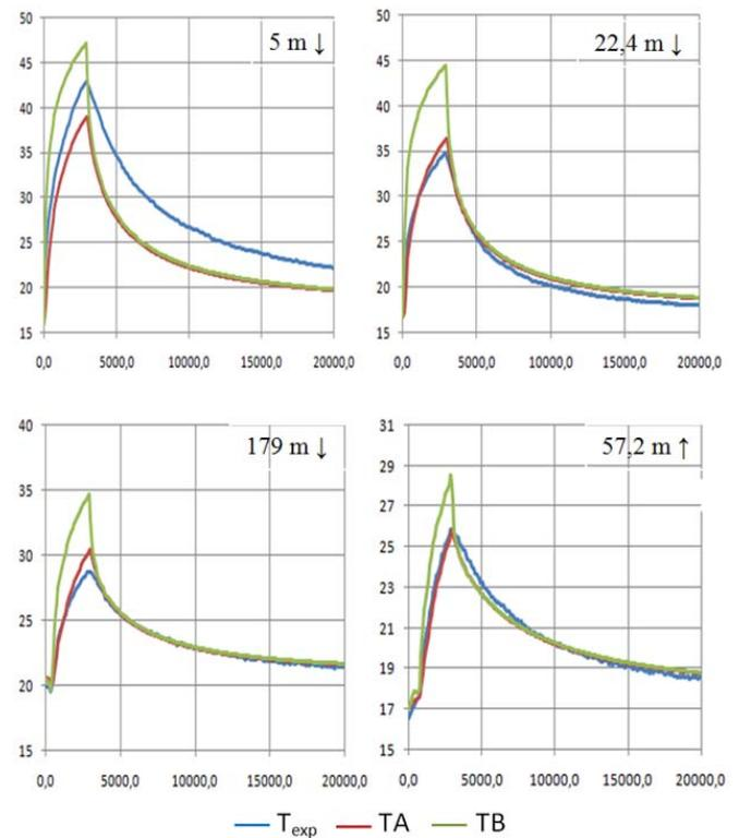
Figure 3: Simulation of the thermal pulse vs. experimental data
