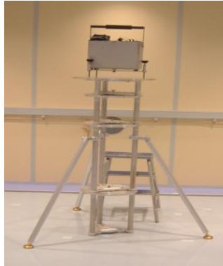
Figure 2.4.3 Set-up of a measurement with a ZLS Burris gravimeter on the enforced tripod
