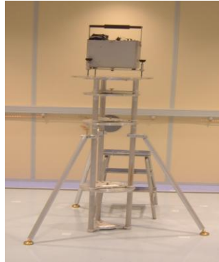
Figure 2.4.3 Set-up of a measurement with a ZLS Burris gravimeter on the enforced tripod
