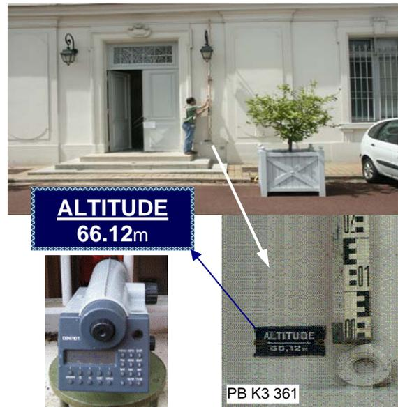
**Figure 3.2.1** The NGF leveling point on the wall of the Observatoire building of BIPM and its value 66.12m in the NGF served as the starting value of the height measurement before the RGC2009. The same point in the new IGN system is numbered P.B.K3-361 with its value 66.4558m in IGN69. The difference between the two systems is:  $IGN69-NGF=+0.3358m$ . The levelling instrument used by IGN was the Zeiss Dini 10
