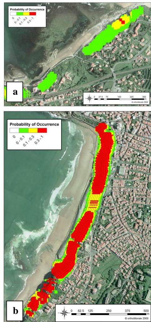
Figure 12 Results of the second modelling for (a) the Parlementia beach and (b) the Côte des Basques cliffs. The displayed probabilities of occurrence correspond much better to the field observations compared to figures 7 and 10.
