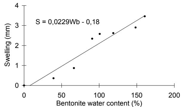
Figure 3. Swelling ( $S$ ) versus water content of the bentonite ( $W_b$ ).
