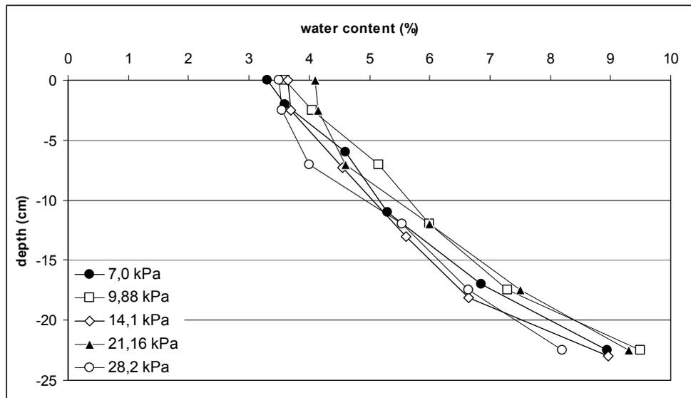
Figure 4. Water content profile in the sand column
