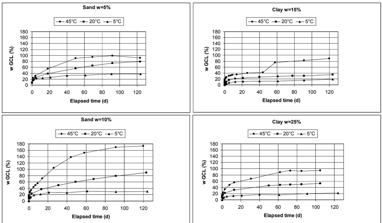
Figure 8. Influence of temperature on GCL hydration
