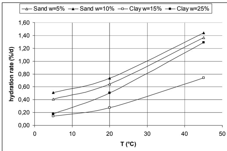
Figure 9. Average hydration rate of GCLs versus temperature.
