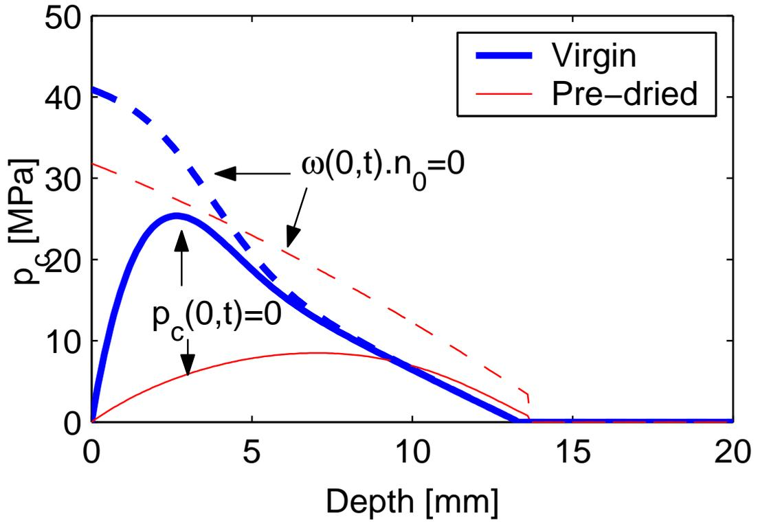
FIG. 7. Liquid and ice pressure profiles for of the virgin and the predried samples at  $t = 2$  hours. The solid line correspond to the  $p_c(0,t) = 0$  boundary condition while the dot line is for the  $\omega(0,t) \cdot n_0 = 0$  one.
