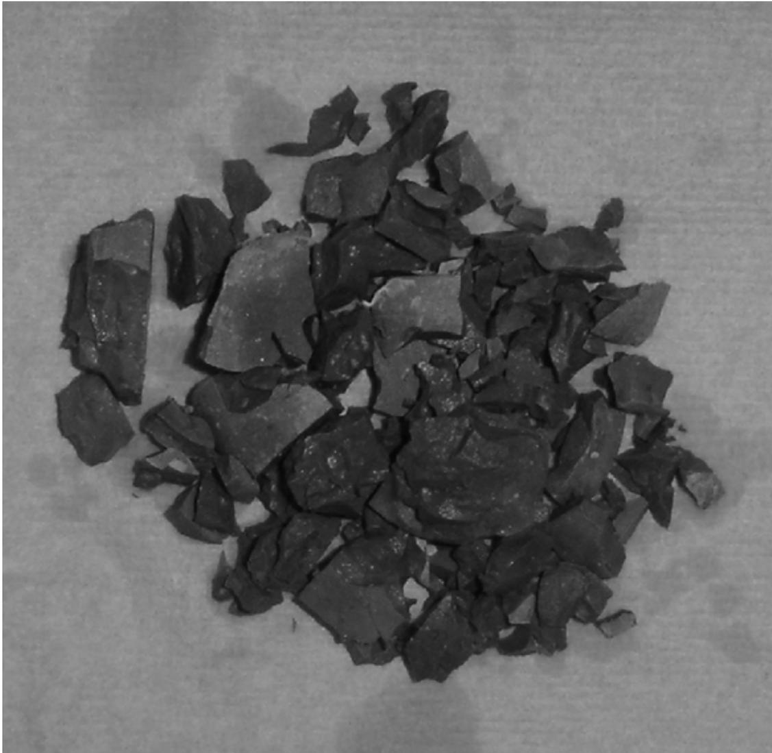
**FIG. 3. Picture of the P4-E-3d cement paste after the first 14 cycles.**
