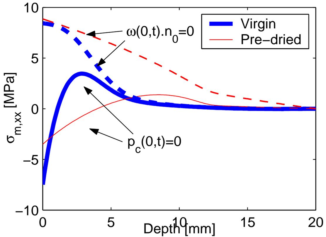
**FIG. 8.**  $\sigma_{m,xx}$  profiles for of the virgin and the predried samples at  $t = 2$  hours. The solid line correspond to the  $p_c(0,t) = 0$  boundary condition while the dot line is for the  $\omega(0,t) \cdot n_0 = 0$  one.
