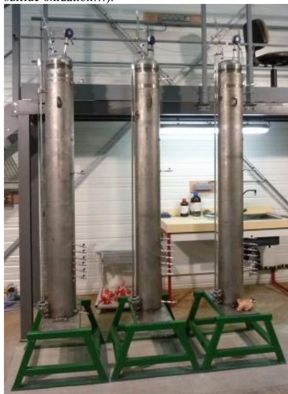
Fig. 1: stainless steel columns use to simulate and monitor sediment/water exchanges during resuspension and settling.
