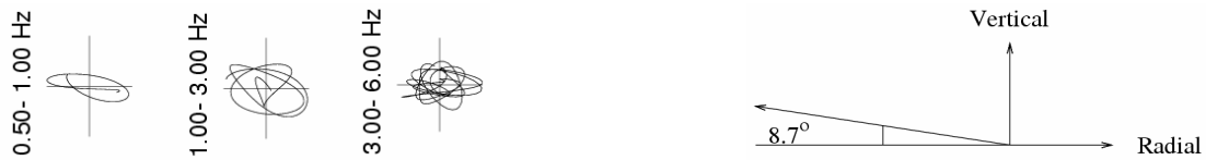
Figure 10: Particle orbits on a vertical plane calculated from borehole accelerograms at the onset of S-wave portion of the main shock. The orbits are calculated from band-pass filtered waves in the frequency range of interest.
