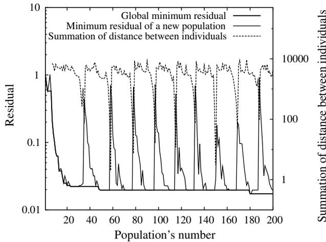
**Figure 19.** Example for an inversion of the evolution of the global minimum residual (bold line), the minimum residual of a new population (thin line), and the summation of distance between individuals (dashed line).
