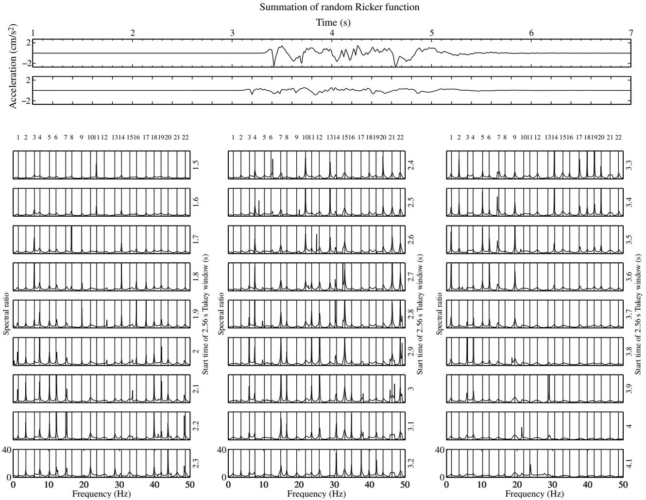
**Figure 13.** Time-dependent spectral ratios analysis performed between downhole and basement waveforms when the input wave is a summation of ten Ricker functions for which pseudofrequency is randomly chosen within the interval 0.5–25 Hz.
