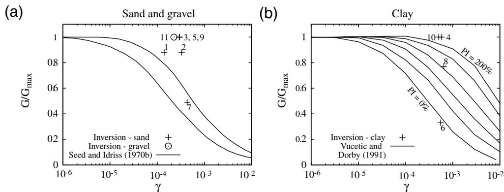
**Figure 24.** (a) Comparison of the strain-dependent characteristics inverted for sand and gravel layers with laboratory test results for sand (Seed and Idriss, 1970b) whose effective vertical stress ranges from 0.05 to 0.5 MPa. (b) Comparison of the strain-dependent characteristics inverted for clay layers with laboratory test results for clay (Vucetic and Dobry, 1991) whose plasticity index (PI) ranges from 0% to 200%. For both panel, numbers indicate layers of Table 3.
