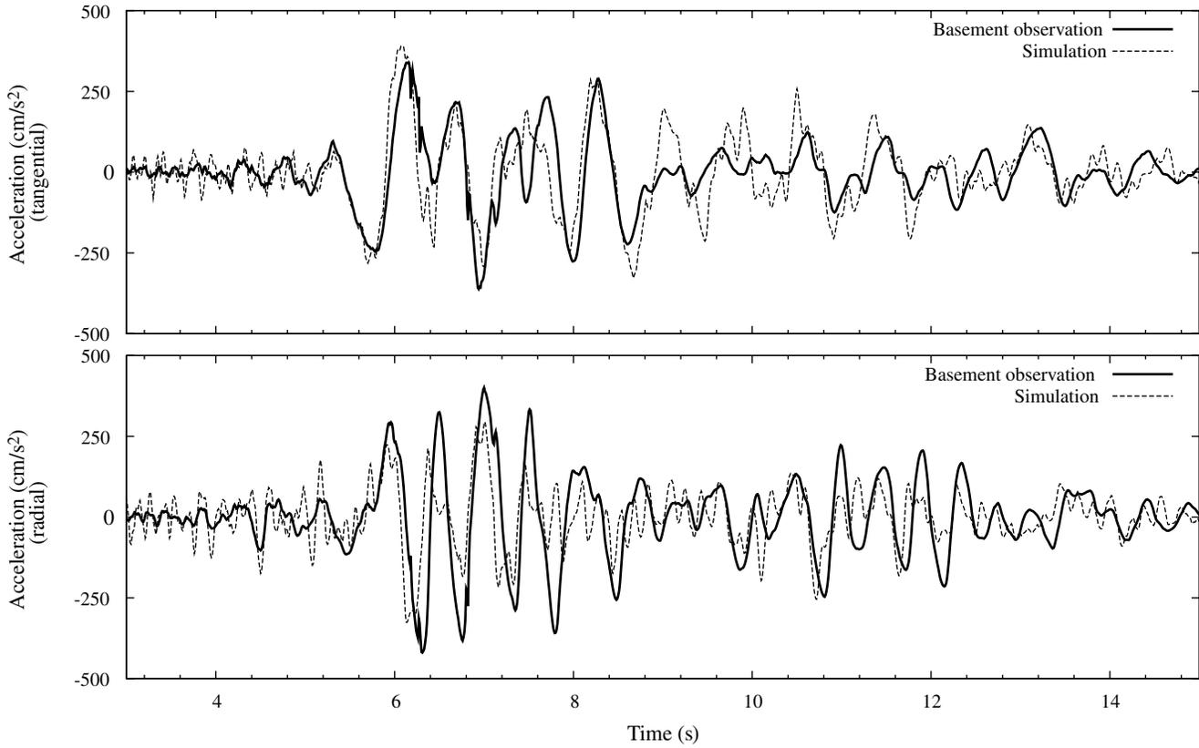
**Figure 22.** Comparison between observed (solid line) and simulated (dashed line) acceleration at the basement in transverse and radial directions.
