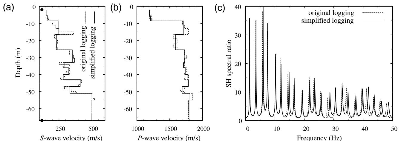
**Figure 9.** (a,b) Original and simplified PS logging. Upper and lower sensors (dots) are located at 2 m and 67 m below the free surface, respectively. (c) *SH* spectral ratio of original and simplified soil column. Low damping has been purposely used to better see the shift of resonant frequencies due to *S*-wave simplification.
