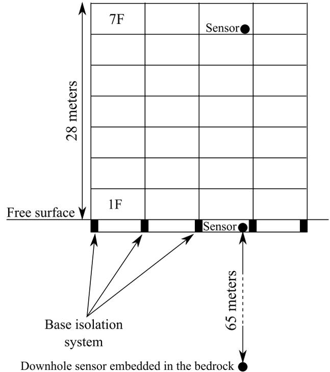
Figure 7. Schematic representation of the system {base-isolated building + borehole station} at the CTI Engineering site. Sensors are represented by circles.
