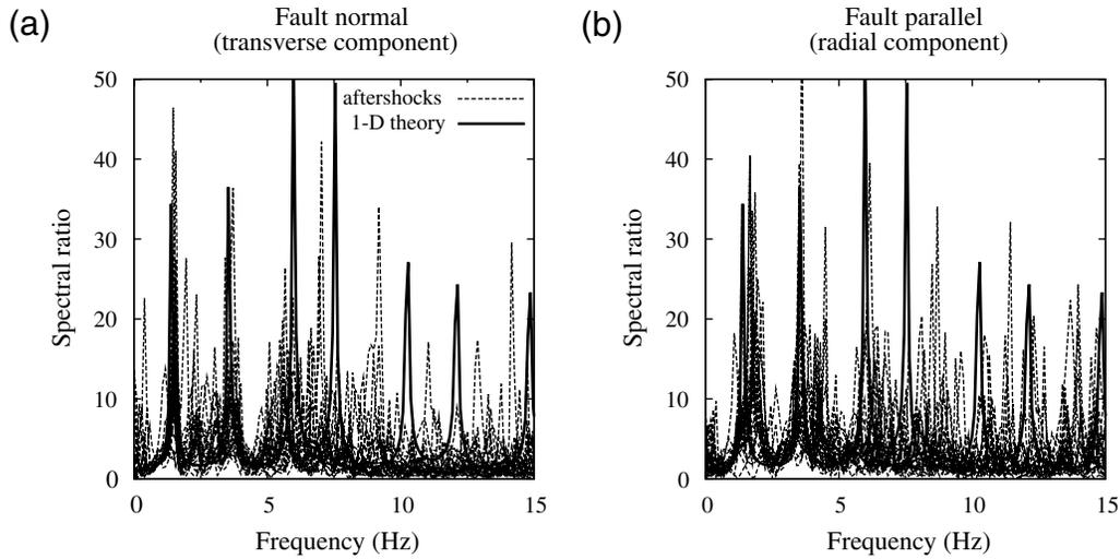
**Figure 10.** (a) Fault-normal spectral ratios. (b) Fault-parallel spectral ratios. Dashed line, spectral ratios performed on the *S*-wave portion of aftershocks chosen by sight; bold solid line, theoretical 1D spectral ratio for a vertically incident *S* wave using the velocity logging. The frequency discretization of spectral ratios is 1/40.96 Hz. A Parzen spectral window of bandwidth 0.1 Hz has been used to slightly smooth observed and theoretical ratios.
