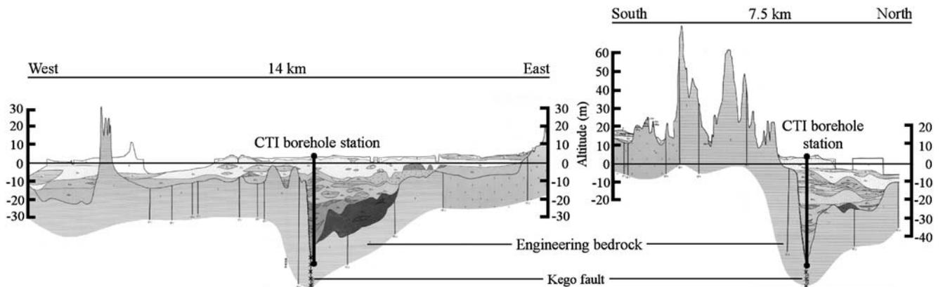
Figure 6. North–south and east–west geologic cross sections located some hundred meters from the CTI borehole station. The vertical axis has been exaggerated. Solid line, borehole station; points along solid line, sensors; crosses, the Kego fault.
