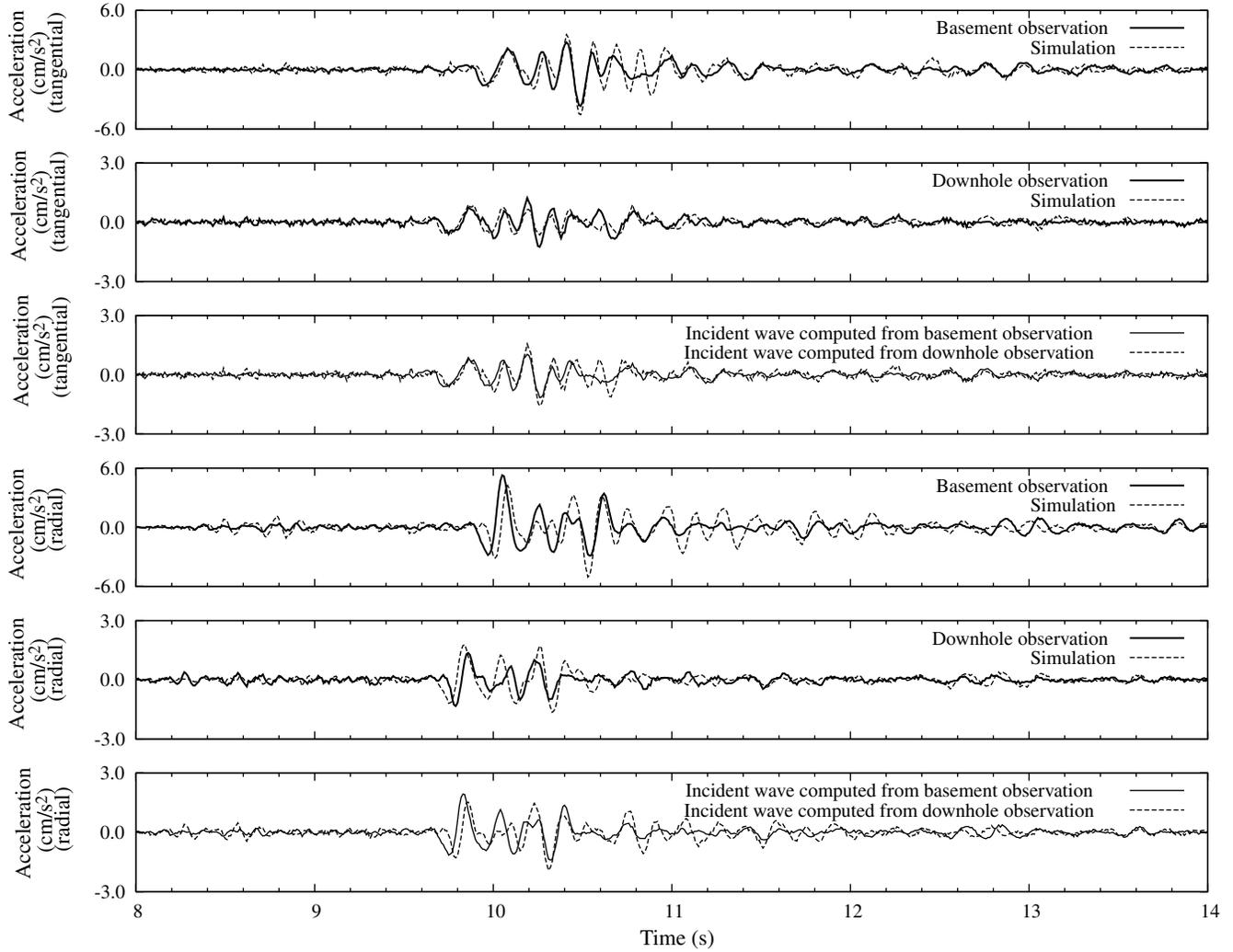
**Figure 15.** Simulations and deconvolutions of EQ11 in transverse and radial directions using  $S$ -wave velocity logging and constant damping factor along the soil column of the form  $h = h_0 f^{-\alpha}$  with  $f$  as the frequency,  $h_0 = 0.13$  and  $\alpha = 0.6$ .
