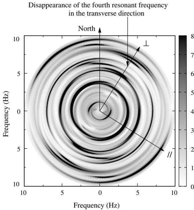
**Figure 17.** The 360° spectral ratio computed during EQ01. Axes denoted by ⊥ and ∥ indicate the fault-normal direction (i.e., transverse component) and the fault-parallel direction (i.e., radial component), respectively.
