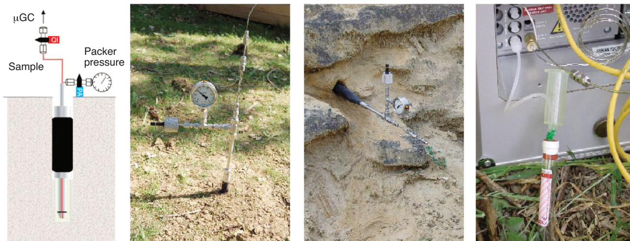
Figure 4 Illustration and photographs of micro-GC sampling.
