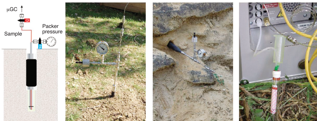
Figure 4 Illustration and photographs of micro-GC sampling.
