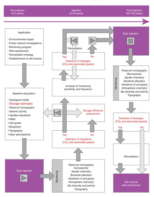
Figure 1 Synoptic diagram of the different steps in monitoring a  ${\rm CO_2}$  storage site.
