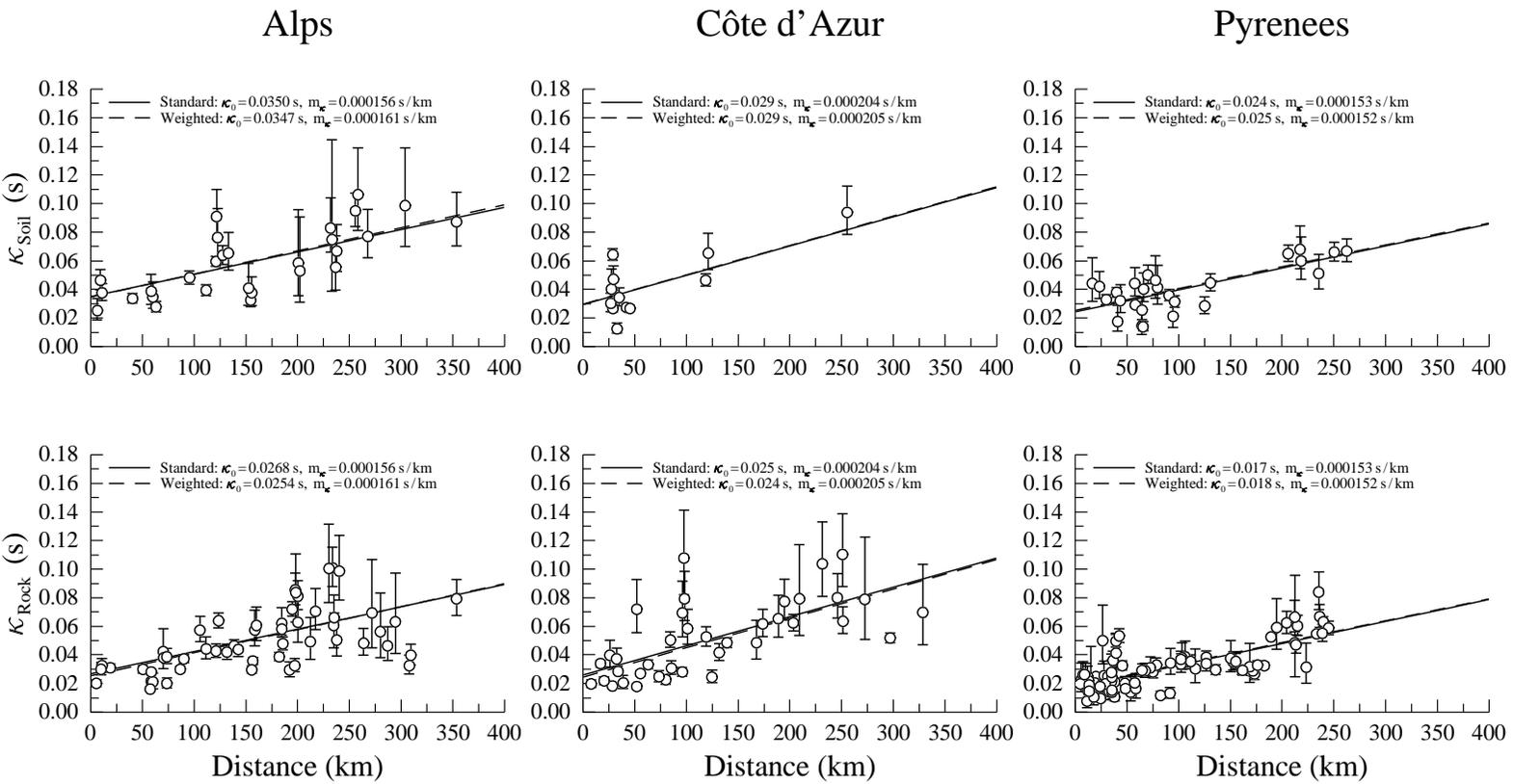
Figure 6: Distance dependence of  $\kappa$  values for three regions in mainland France. The top plots present the results for stations located on soil. The bottom plots show the results for stations located on rock.
