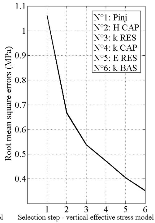
Fig. 3 - Evolution of the Root Mean Square Error during the selection procedure of the most influential input variables for the response surface model respectively associated with the horizontal (left figure) and the vertical (right figure) effective stress.
