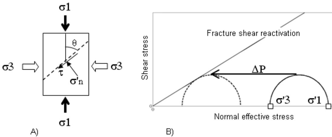
Figure 2: A) Stress components acting on a fracture plane in a rock sample, B) change in the stress state due to increase of the pore pressure in the Mohr diagram
