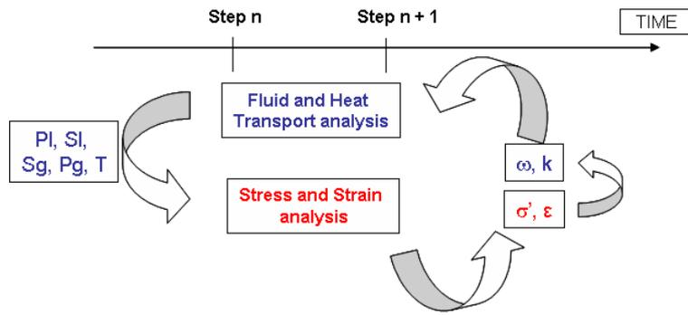
Figure 1: Schematic view of sequentially linking specialized codes respectively in fluid and heat transport analysis (TOUGH2 from LNBL) and stress and strain analysis (Code\_Aster from EdF)
