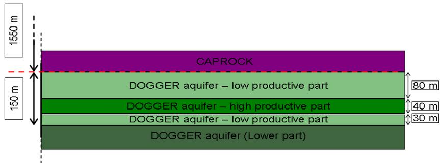
Figure 4: Schematic view of the Dogger reservoir
