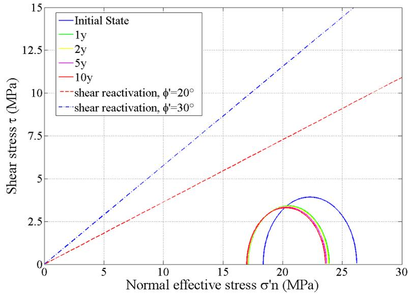
Figure 11: Evolution of effective stress state (Mohr diagram) at the interface between the caprock and the reservoir layer (depth = -1550m) in the injection zone (radial distance <100m) during injection and comparison with shear reactivation criteria
