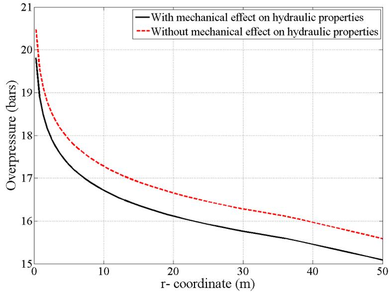
Figure 5: Comparison of pore pressure profile between a one dimensional axisymmetric hydromechanical model (based on Andre *et al.*, 2007) taking in to account the mechanical effect on hydraulic properties (coupling relationship of David *et al.*, 2001), straight black line, and a model without such mechanical effect (dashed red line).
