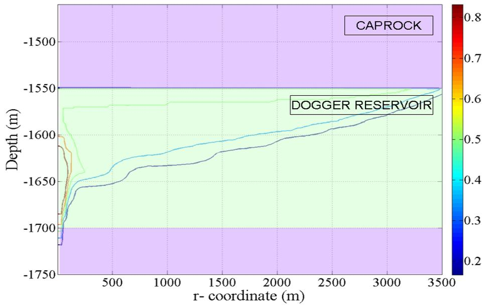
Figure 7: Gas saturation field after 10 years of storage
