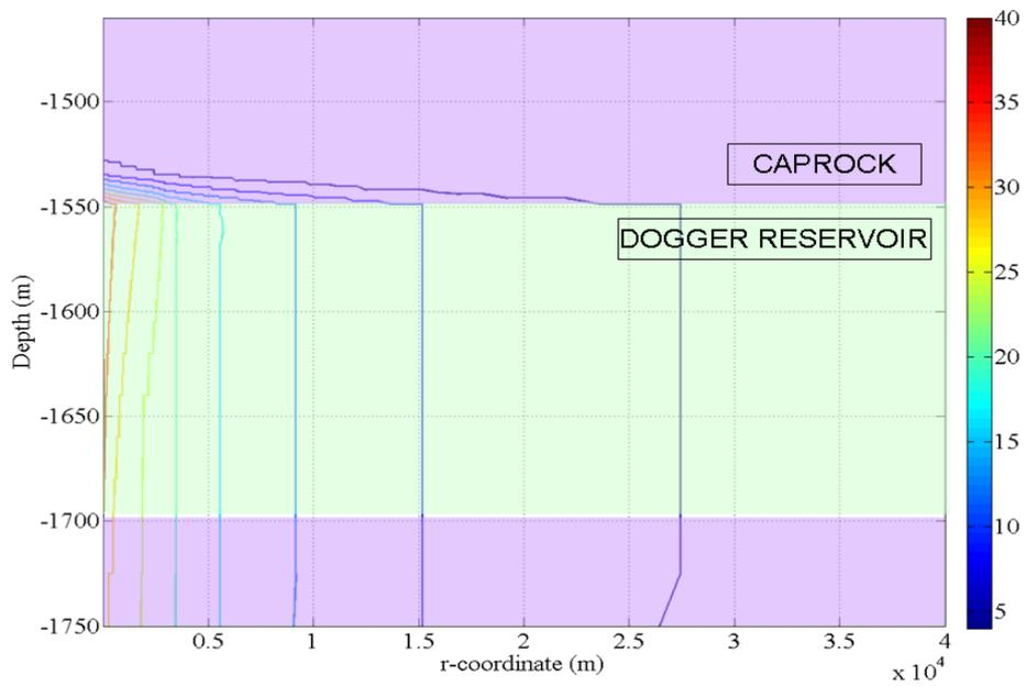
Figure 8: Overpressure field (bars) after 10 years of injection
