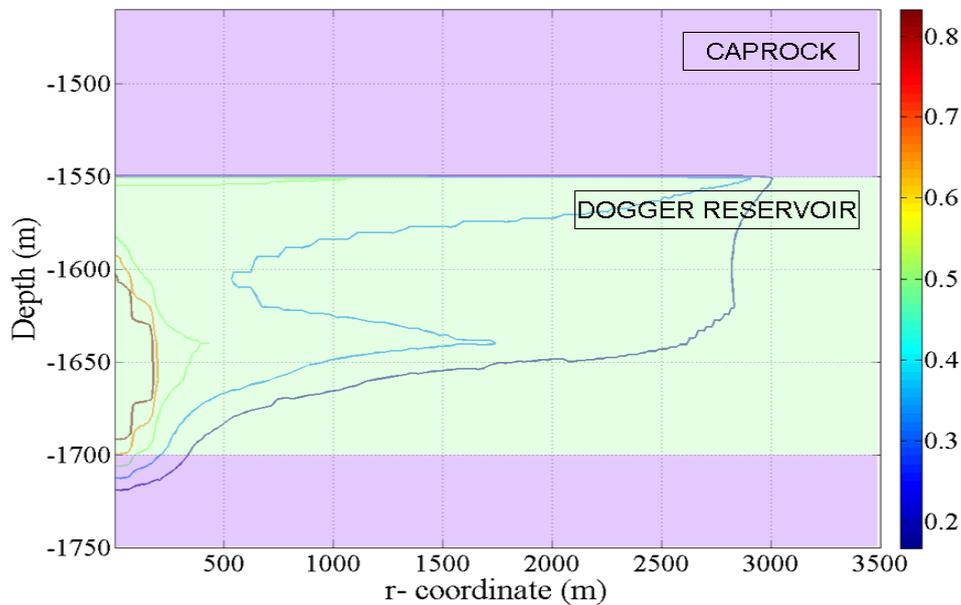
Figure 6: Gas saturation field after 10 years of injection
