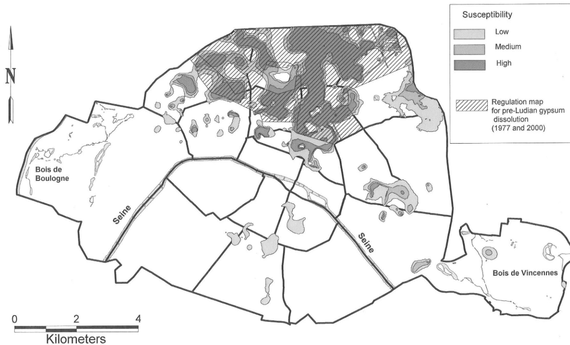
Fig. 17: Comparison between results obtained on Brackish Marl and Limestone formation and the regulation map.
