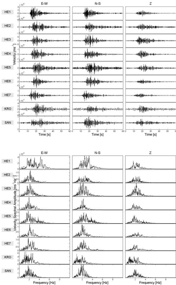
**Figure 5 - Long-period earthquake on 1st July 2006 at Hengill. (top) 60 seconds of unfiltered signal (bottom) frequency spectra. Note that the frequency content at all stations is similar. We believe it is a source effect rather than a path effect.**
