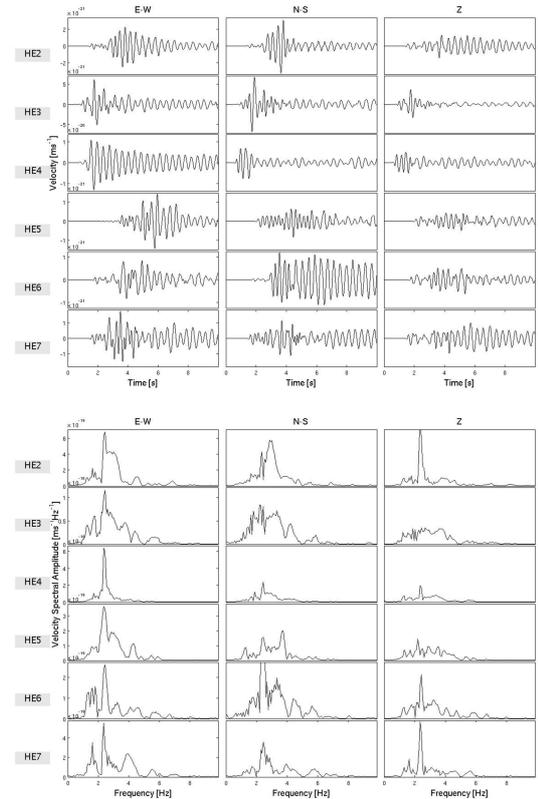
**Figure 6 – Synthetic long-period earthquake modeled using 3D finite-difference including velocity model and topography of Hengill. No attenuation is included in this case. The grid spacing is 100 m in horizontal direction and 50 m in vertical direction. Time step is 0.003 s. (top) 10 s of unfiltered signal (bottom) frequency spectra.**
