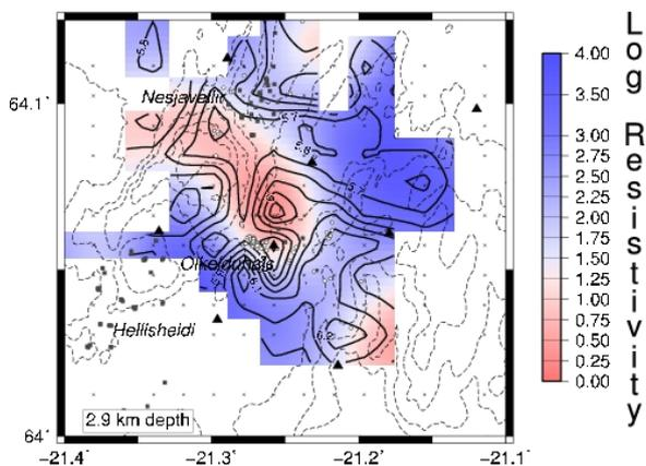
**Figure 8 – Comparison between the resistivity model obtained from the inversion of TEM and magnetotelluric data (Arnasson et al., 2009) and the P-wave velocity model (continuous lines, contour interval 0.1 km/s) obtained from the tomography of broadband observations at Hengill geothermal system at 2900 m depth. Black triangles are broadband station locations.**
