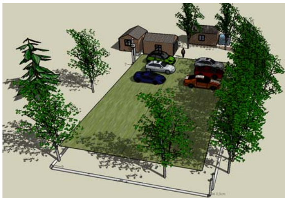
Figure 2: View of the 4 different sectors of horizontal ground heat exchangers
